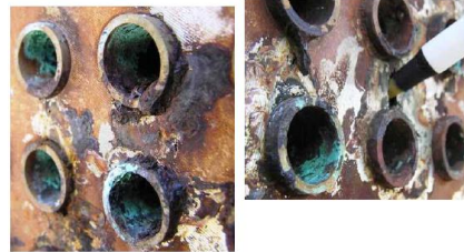
Figure 3. Tubesheet after hydro blasting. Note severe pitting and under deposits corrosion on the tubesheet and corrosion products (greenish) inside tubes. The tubesheet corrosion may have been aggravated due to galvanic effect of tube material.
